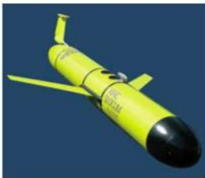
FIGURE 6.19 Submersible robotic gliders, such as the one in this photo, are used to collect physical measurements in ocean water, such as temperature.
